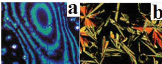
Figure 3. Microphotographs obtained in between the crossed polars. (a) Co-existent biphasic region of nematic (N + I) phase (250X). (b) Co-existent biphasic region of columnar smectic (C + I) phase (250X).
